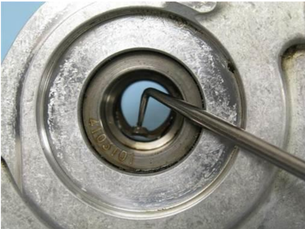
Note intake rod seal on intake cylinder just inside cylinder inboard side. Note: Picture is of different vanos and shows burnt sludge buildup.
