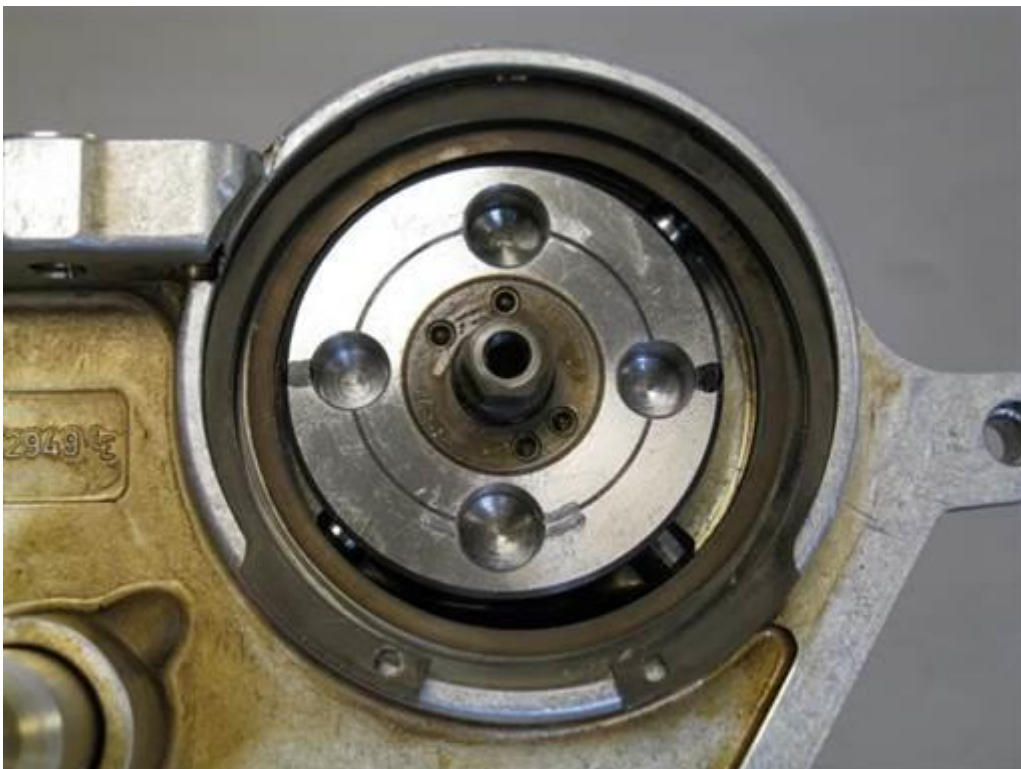
Initially insert retaining ring in oil pump housing.
