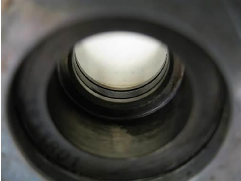
Note intake rod seal on intake cylinder just inside cylinder inboard side. Note: Picture is of different vanos and shows burnt sludge buildup.
