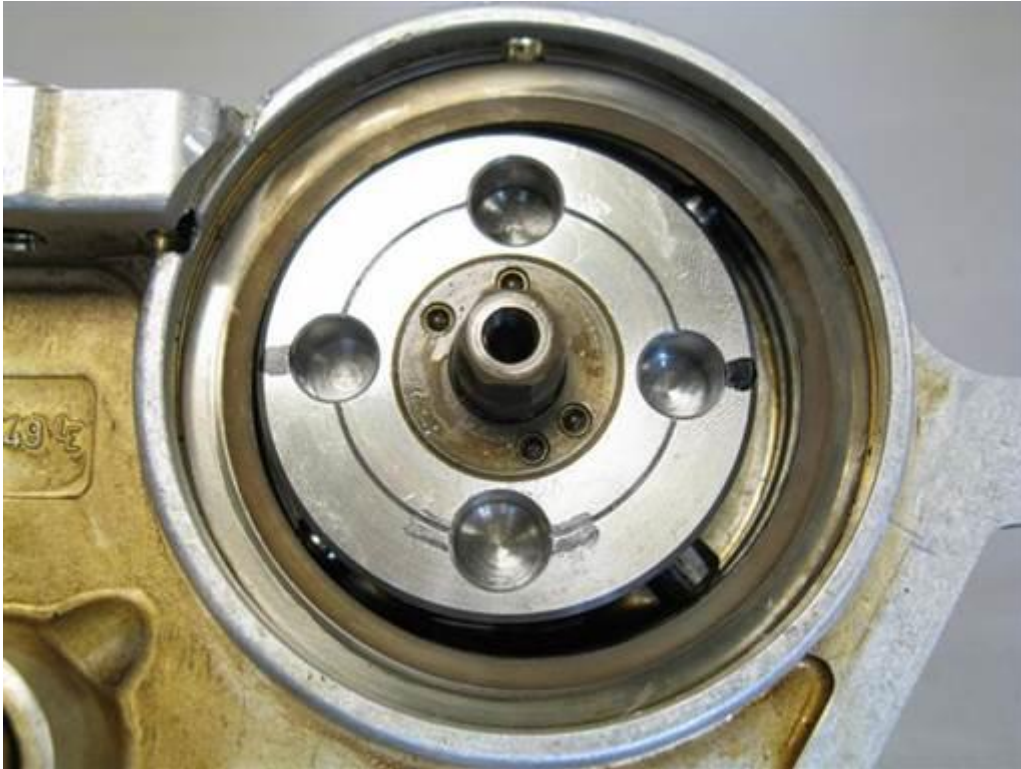
Install retaining washer in oil pump housing.
